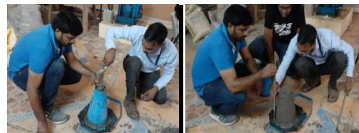
Fig.-3 Slump test of concrete
