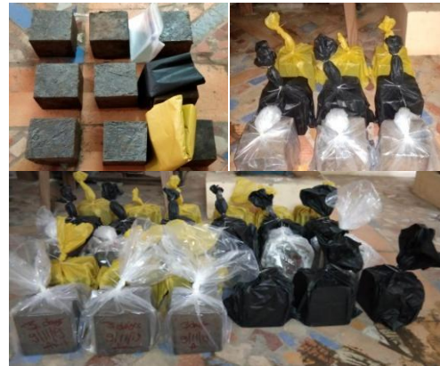
Fig.-7 Concrete cube are cover by 3 different colour polythene for curing
