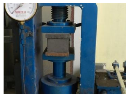
Figure-8 Testing of cubes for compressive strength
