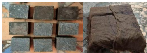
Fig.-6 Concrete cube are cure by wet jute bag for 30 minutes before cover by polythene
