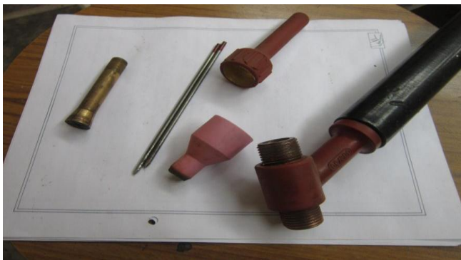
Fig 2: GTAW Torch with collet, electrode, ceramic cup handle.
