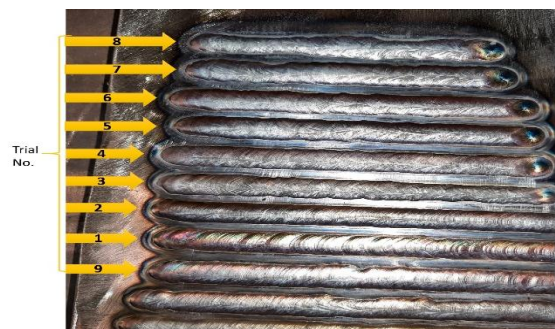
Fig. 6- L9 trials bead profiles according to Taguchi's OA
