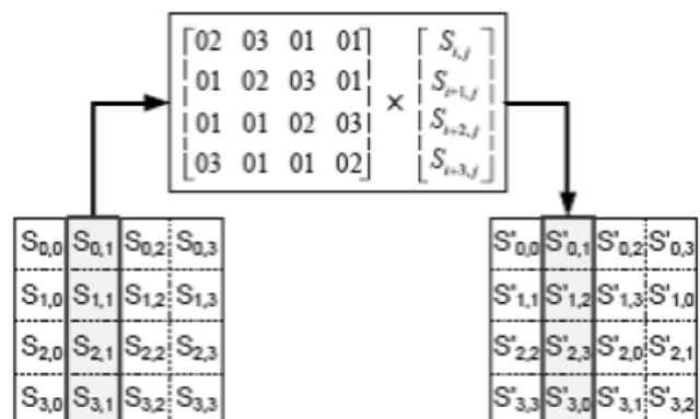
Fig.6 Mix Column Process
